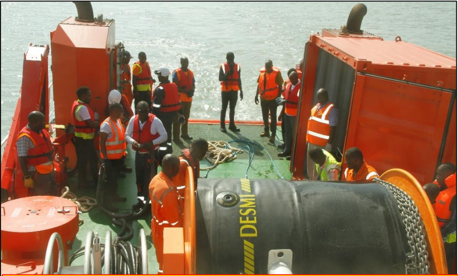
Boom fully recovered from the water and back on its reel
