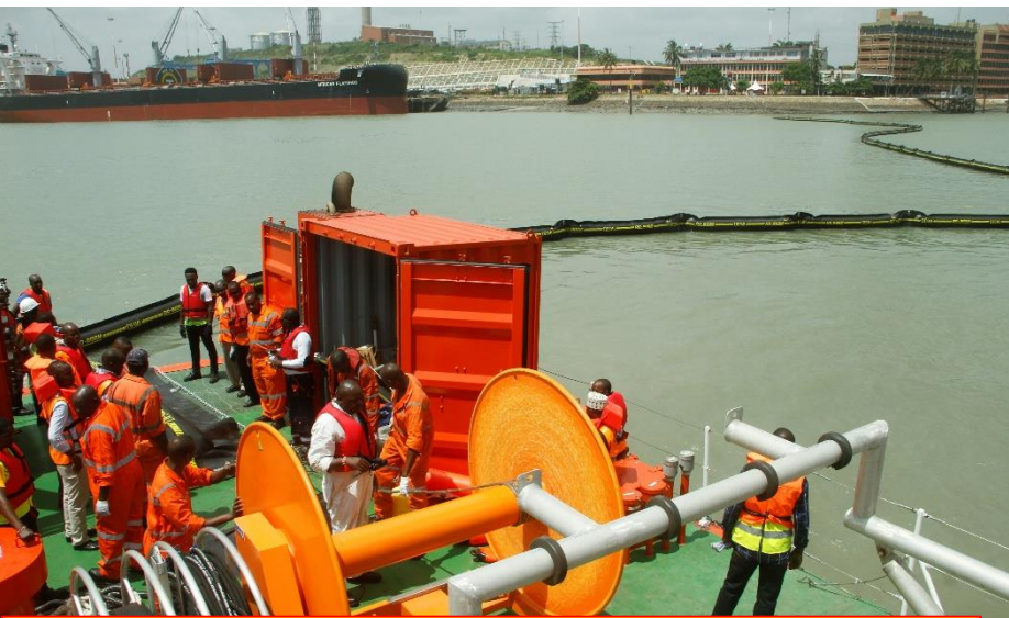
B&S Team complete roll out of the entire boom from its reel
