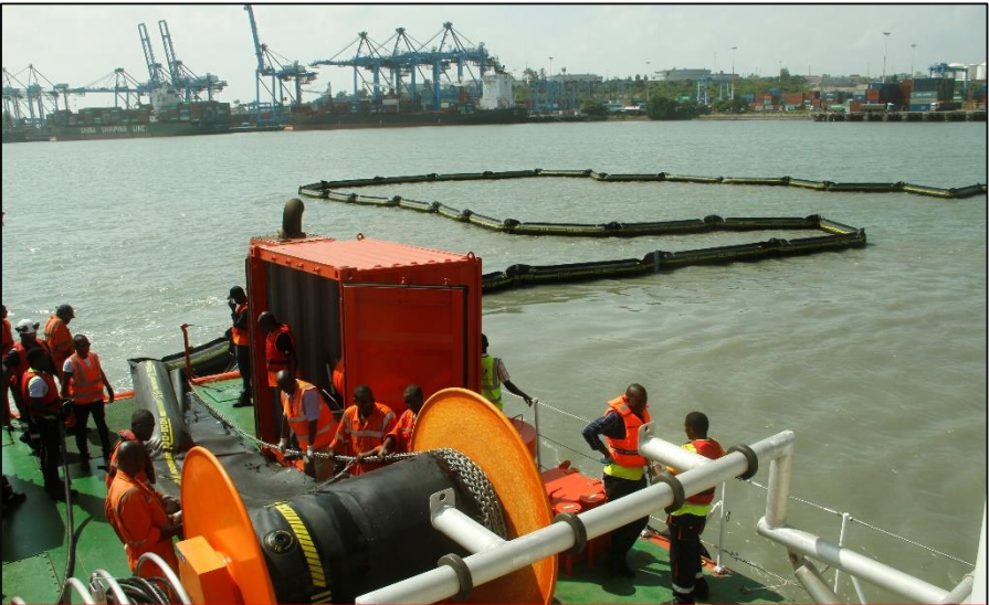
Retrieval of the boom in process
