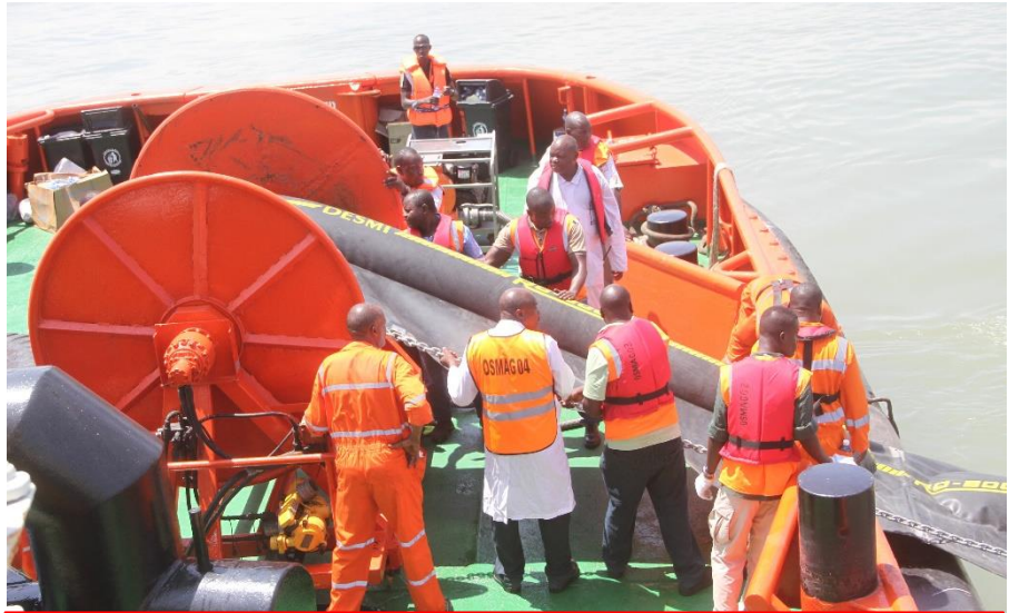
Booming Team manually deploy the boom onto the water
