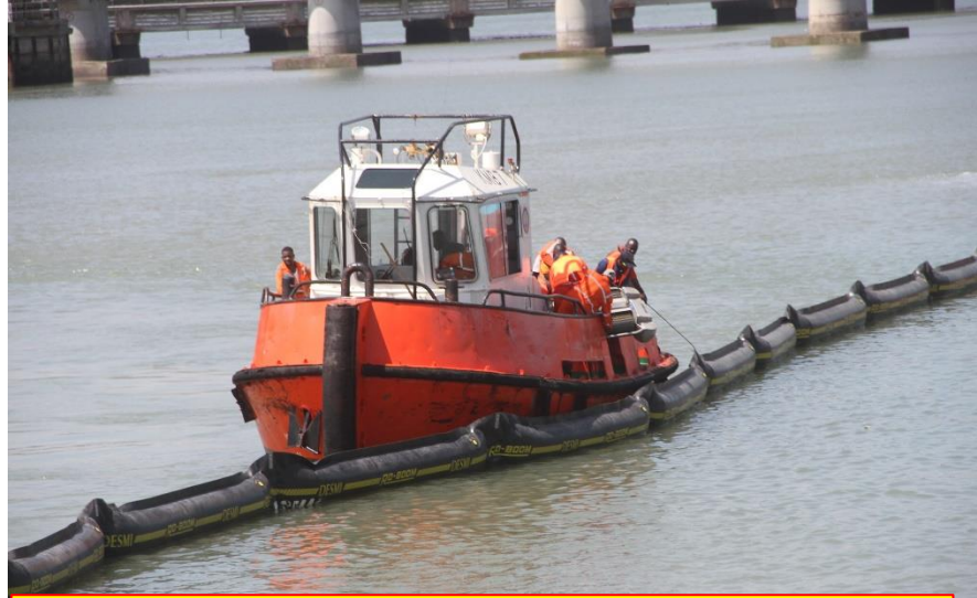
Skimming Team deploying the skimming unit onto the water
