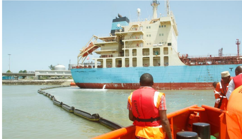
Boom successfully deployed aside the vessel M/T Kristen Maersk
