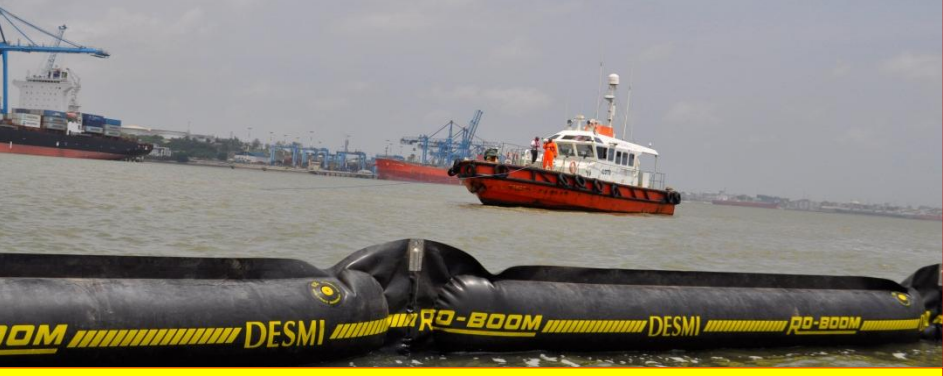
CLOSE UP VIEW OF THE DEPLOYED BOOM
