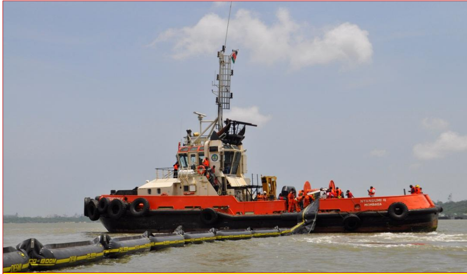
TUG NYANGUMI DEPLOYING LAST BOOM SECTION
