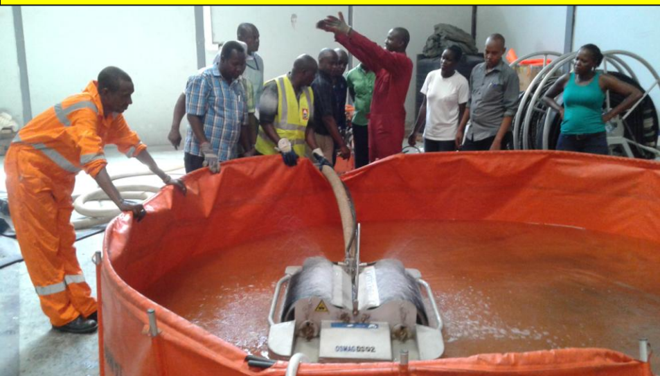
MR GITAU MUHIA OF OSMAG TRAINS A GROUP ON THE OPERATION OF A SKIMMER
